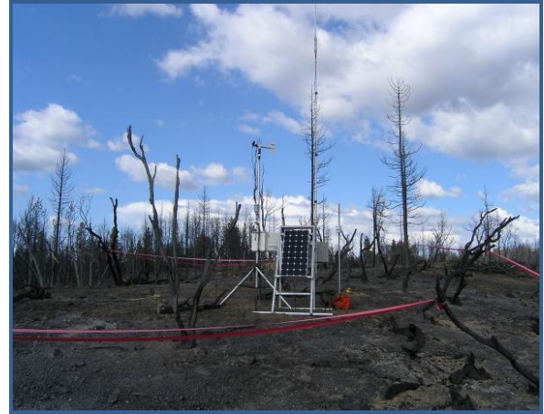
Figure 21. This photograph shows the portable weather station deployed within the study area.
