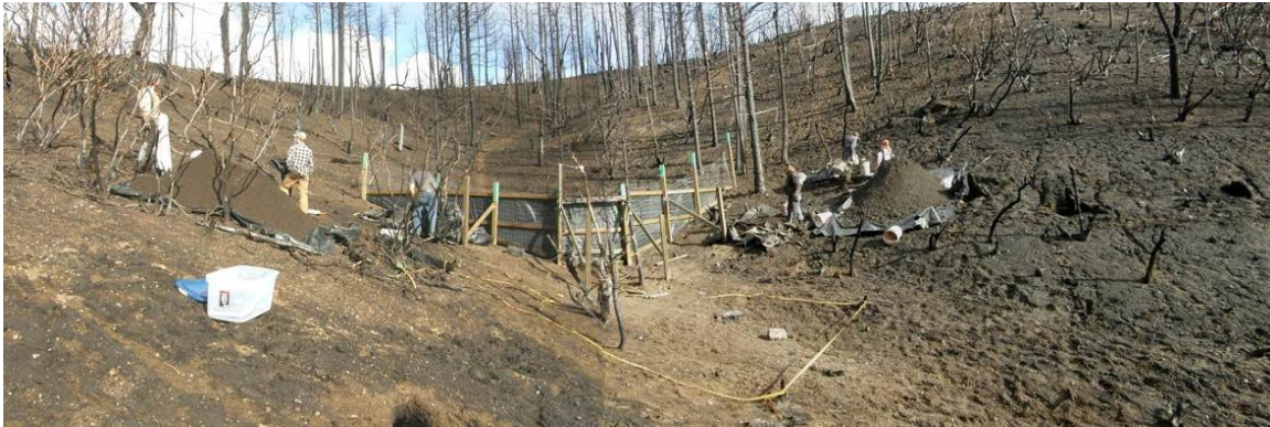
Figure 19. This photograph shows an upslope view during a clean-out. Weighed sediment is piled on the sides and downslope of the fence. This image is of control site 8. The sediment piled to the sides was removed during the first round of cleanouts in December 2012. The sediment pictured accumulated during the first 3 months following fire containment. Note that on the control sites rill erosion features began forming on the burned hill slopes immediately after rainfall events. At this control site a main channel has begun to form; it shows as the lighter brown streak extending uphill from the fence through the middle of the swale.
