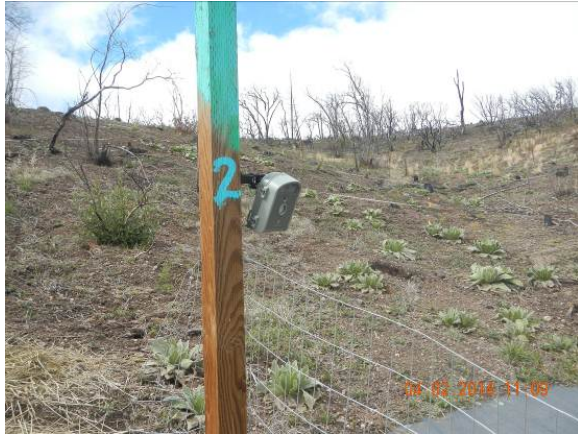
Figure 22. Time-lapse cameras were mounted on the wing walls of the sediment fences to document water and sediment accumulation during rain events.
